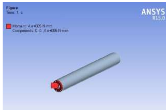
Fig. 10: Applying moment of 400Nm to the Shaft with Ribs
