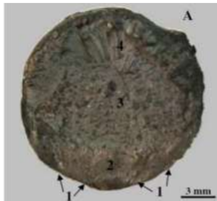
Fig. 3 Fatigue Crack Propagation
