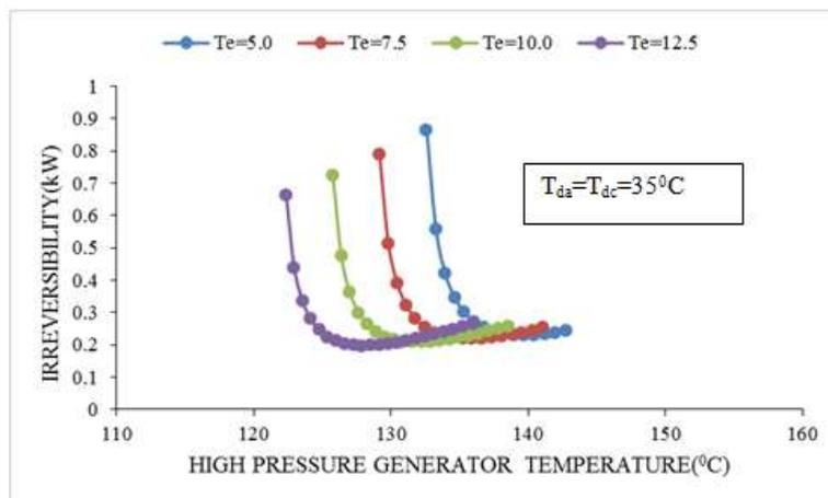
**Fig. 11** Variations in irreversibility of double effect series flow cycles with high pressure generator temperature at secondary condenser temperature 90°C.
