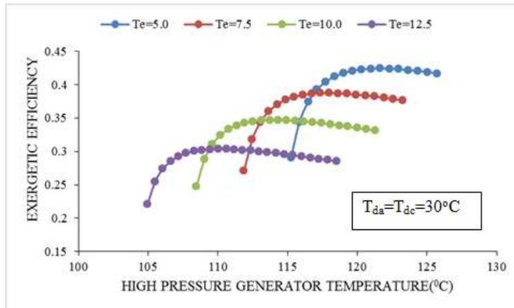
**Fig. 3** Variations in exergetic efficiency of double effect series flow cycles with high pressure generator temperature at secondary condenser temperature 80 °C.
