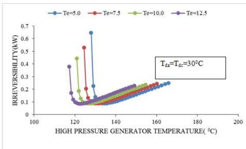
Fig. 14 Variations in irreversibility of double effect parallel flow cycles with high pressure generator temperature at secondary condenser temperature 90°C.
