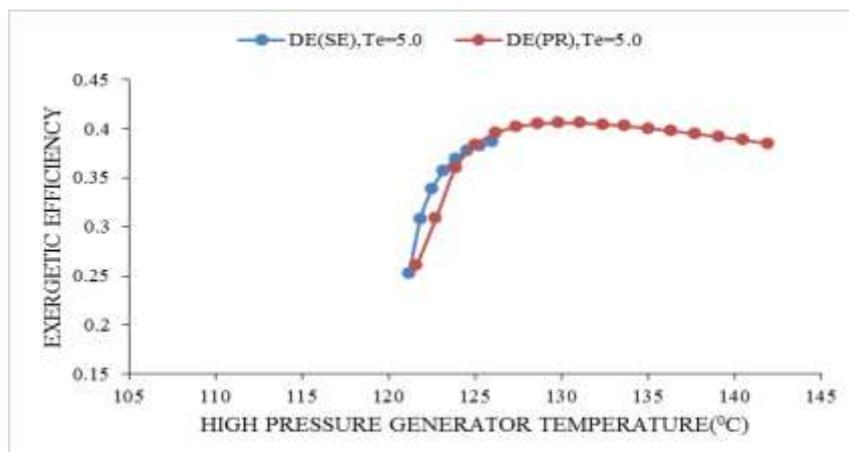
**Fig 5** Variation in exergetic efficiency of double effect (series and parallel flow) cycle with high pressure generator temperature at  $T_e = 5.0^\circ\text{C}$  and  $T_{da} = T_{dc} = 35^\circ\text{C}$
