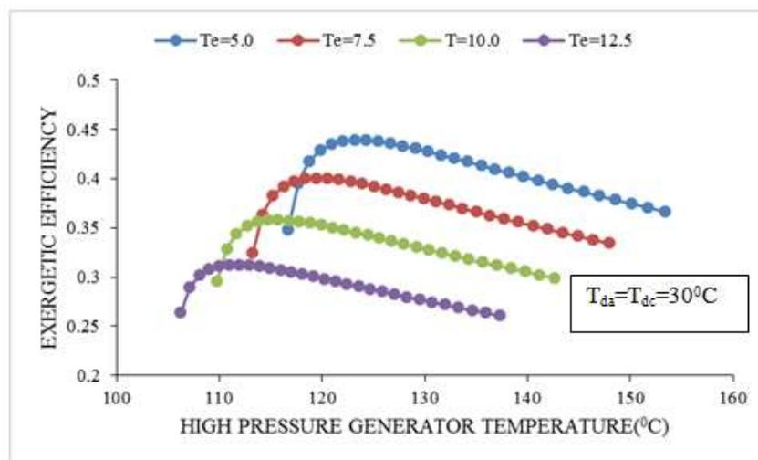
**Fig. 4** Variations in exergetic efficiency of double effect parallel flow cycles with high pressure generator temperature at secondary condenser temperature 80 °C.
