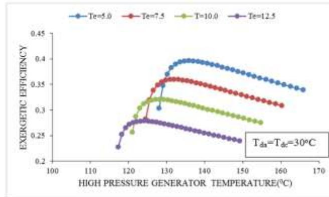
**Fig. 6** Variations in exergetic efficiency of double effect parallel flow cycles with high pressure generator temperature at secondary condenser temperature 90 °C.
