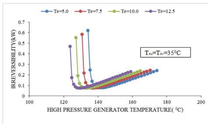
Fig. 15 Variations in irreversibility of double effect parallel flow cycles with high pressure generator temperature at secondary condenser temperature 90°C.
