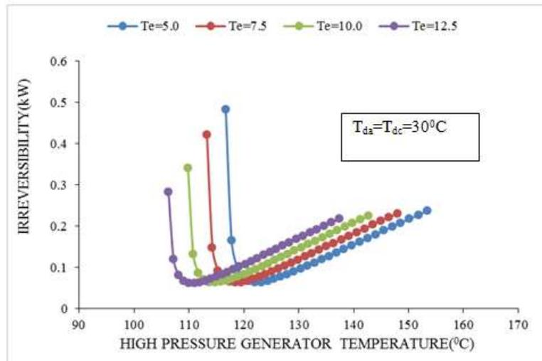
Fig. 12 Variations in irreversibility of double effect parallel flow cycles with high pressure generator temperature at secondary condenser temperature 80°C.
