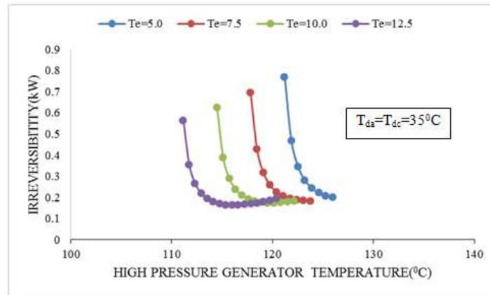
**Fig. 9** Variations in irreversibility of double effect series flow cycles with high pressure generator temperature at secondary condenser temperature 80 °C.
