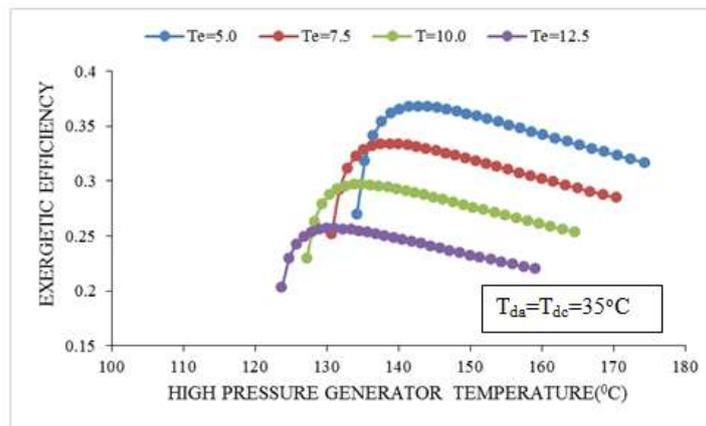
**Fig. 7** Variations in exergetic efficiency of double effect parallel flow cycles with high pressure generator temperature at secondary condenser temperature 90 °C.
