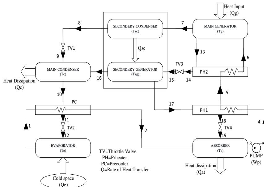
**Fig. 1: Double Effect Series Flow Vapour Absorption Refrigeration System**
