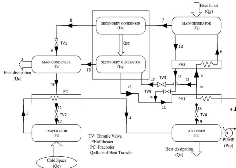
**Fig. 2: Double Effect Parallel Flow Vapour Absorption Refrigeration System**
