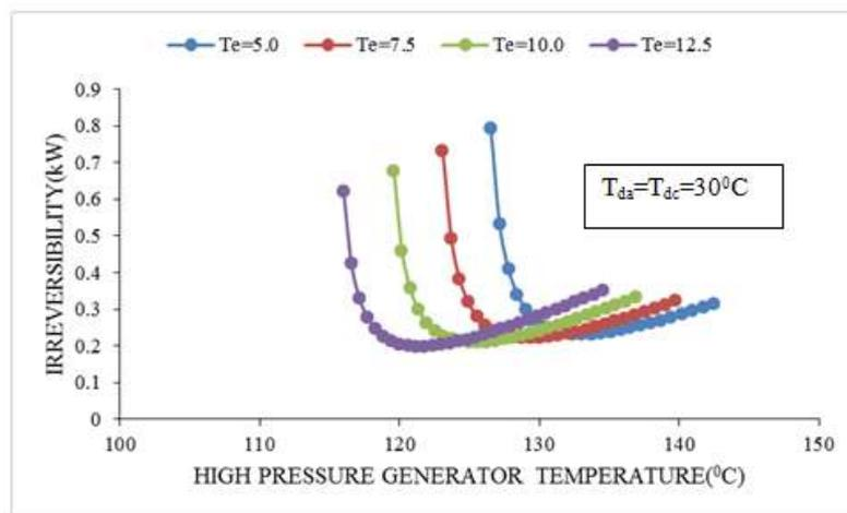
**Fig. 10** Variations in irreversibility of double effect series flow cycles with high pressure generator temperature at secondary condenser temperature 90°C.
