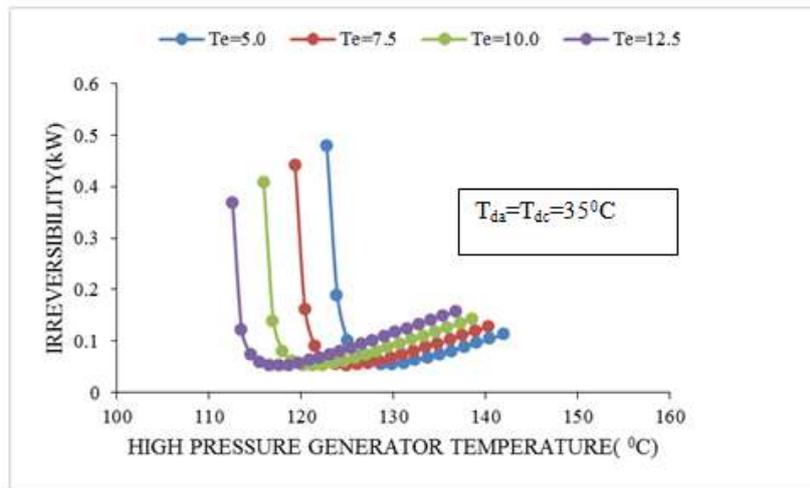
Fig. 13 Variations in irreversibility of double effect parallel flow cycles with high pressure generator temperature at secondary condenser temperature 80 °C.
