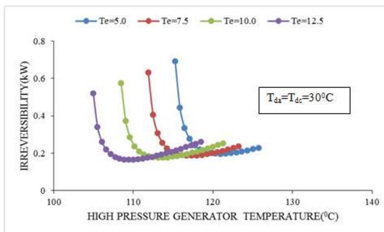
**Fig. 8** Variations in irreversibility of double effect series flow cycles with high pressure generator temperature at secondary condenser temperature 80 °C.
