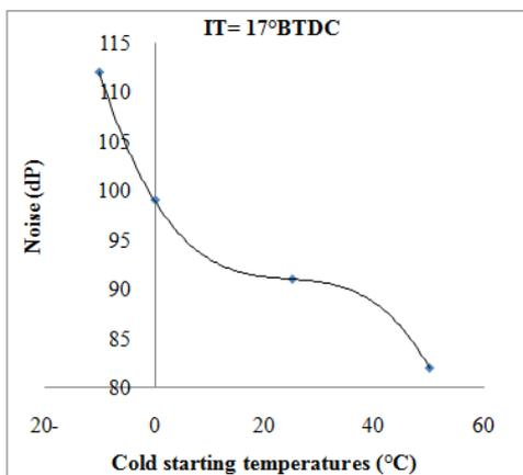
**Fig. 5,** variable starting temperatures effect on emitted engine noise
