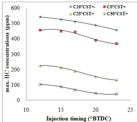
**Fig. 7,** Injection timing effect on engine maximum emitted HC concentrations
