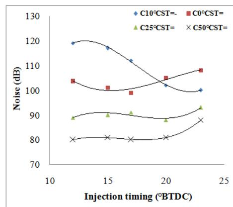
**Fig. 10,** Injection timing effect on emitted engine noise
