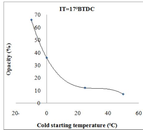
**Fig. 4,** variable starting temperatures effect on emitted engine smoke opacity
