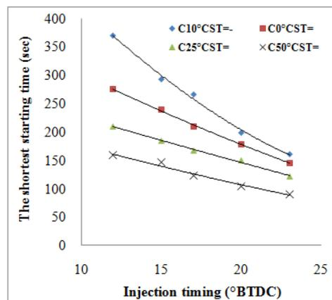
**Fig. 6,** Injection timing effect on the engine starting time
