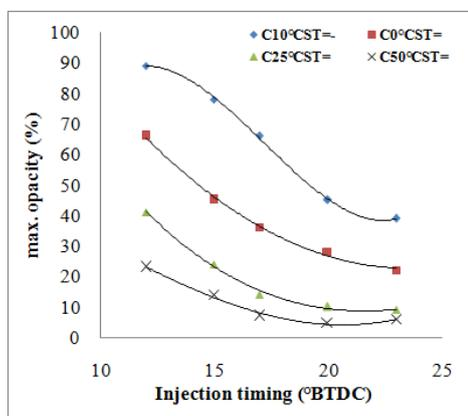
**Fig. 9,** Injection timing effect on emitted engine smoke opacity
