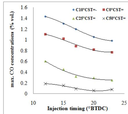
**Fig. 8,** Injection timing effect on emitted engine CO concentrations
