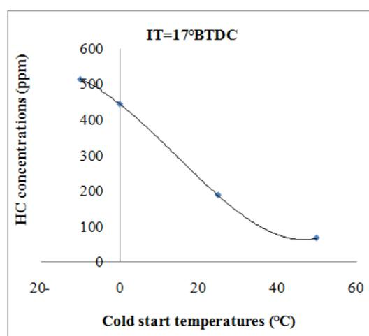
**Fig. 2**, variable starting temperatures effect on emitted engine HC concentrations
