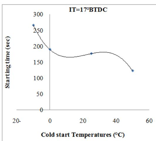
**Fig.1**, variable starting temperatures effect on engine starting time
