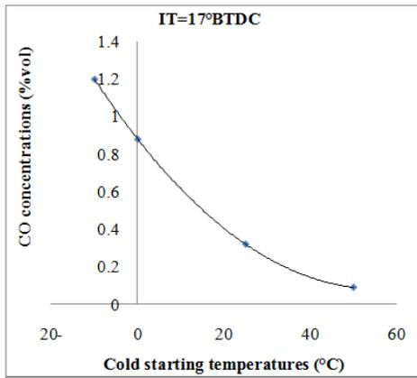
**Fig. 3,** variable starting temperatures effect on emitted engine CO concentrations
