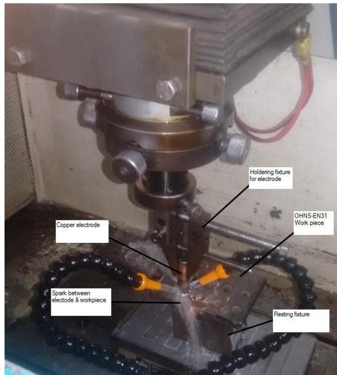
**Fig. 19** EDM machine View
