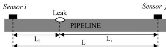
Figure 4: Input from two sensors with the pipeline
