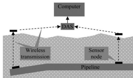
Figure 7: WSN checking framework for checking underground pipeline leak.
