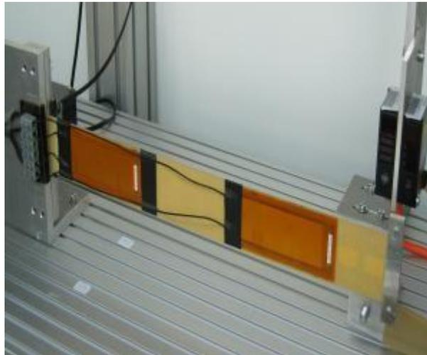
Figure1: Flexible Macro Fiber Composite (MFC) sensors
