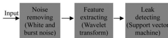
Figure 3: Identification technique in 3 stages
