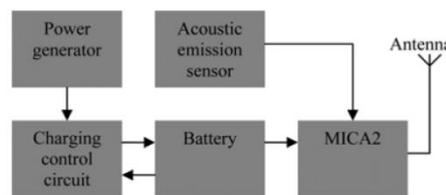
Figure 6: hubs of leakage observing frameworks for underground pipelines
