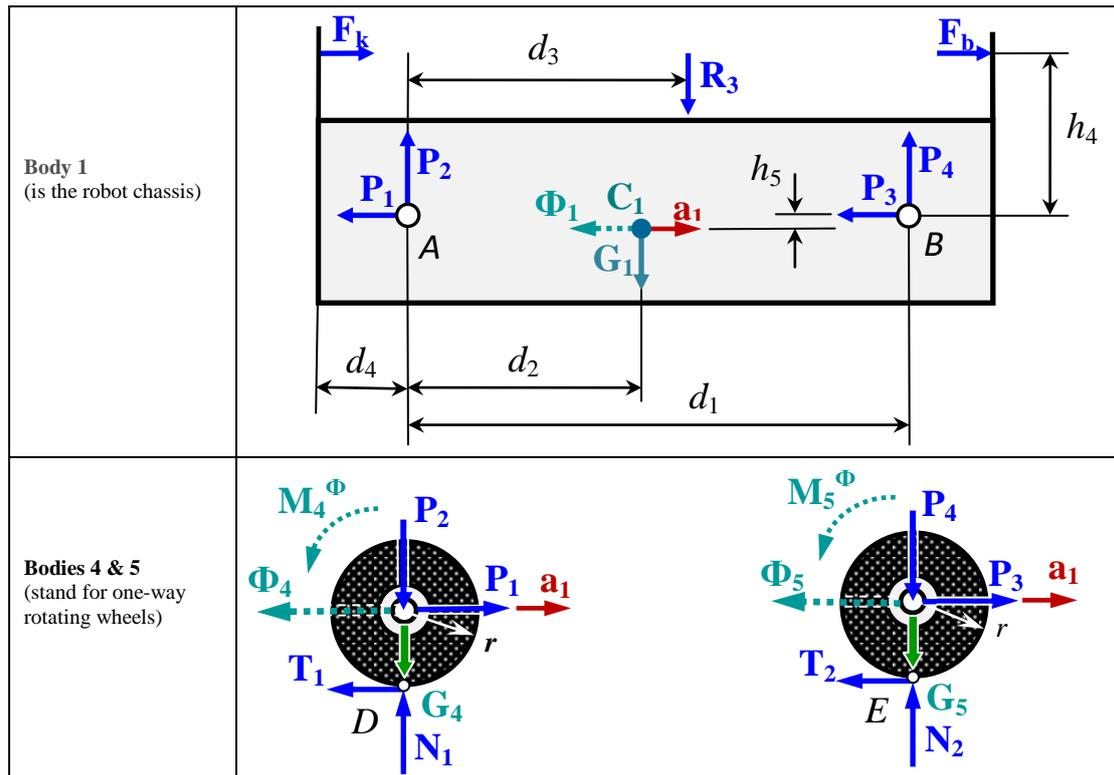
In case that all the wheels are rolling without slipping then the friction forces between them and the contact surface are very small (pure rolling friction) or in the border case they may be equal to the maximum value of the corresponding friction force  $T_j^*$ , which is defined as:
