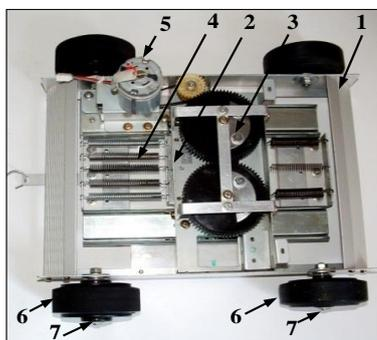
Fig. 1 displays the top view of the prototype robot, where: 1 is the outer frame (body1), 2 - inner frame (body2), 3 contra-rotating eccentric masses (body3), 4 - spring system, 5 - DC motor, 6 - one-way rotating wheels, 7 - one-way rotating bearings.
