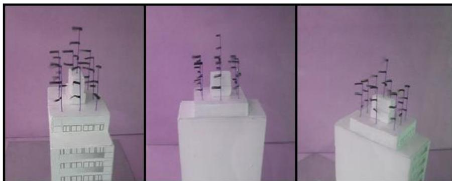
**Figure 8:** Tufts indicating turbulence at different heights on the roof of the building B. The wind in all pictures ran from right to left.
