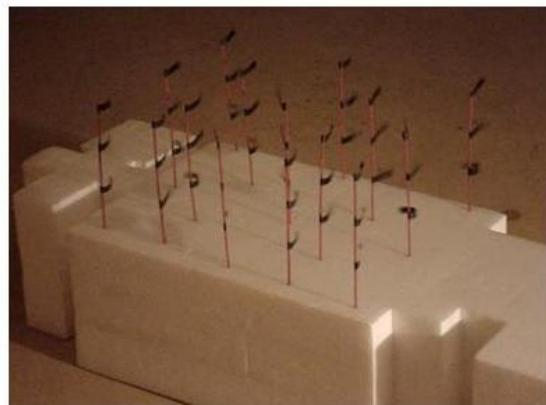
(d) Wind SW direction, tufts to 2.5 to 5 and 7.5 m
