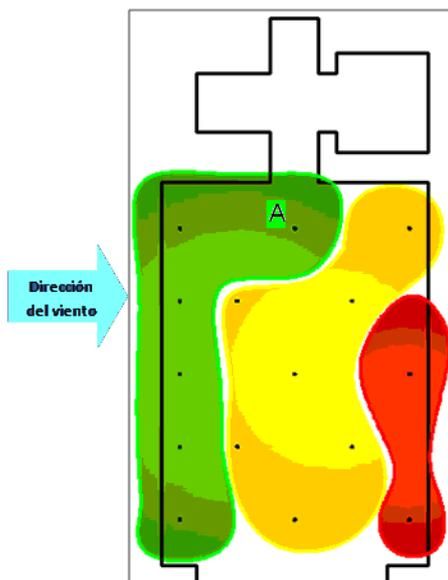
**Figure 6:** Zoning ceiling where it is advisable to install wind turbines. (Green) and stable maximum winds (yellow) turbulent (red) and effect of the turbulent wake.
