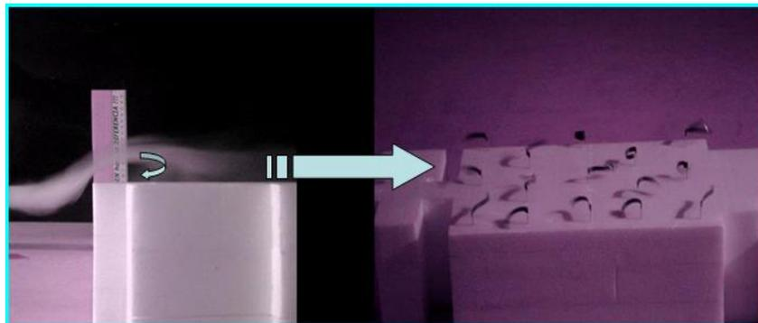
**Figure 1:** The trace of smoke indicates the bubble that is formed in the ceiling of the building, and the tufts show the turbulence of the zone near to the ceiling.
