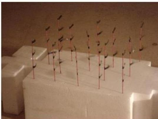
(c) Wind Direction WSW, tufts to 2.5; 5 and 7.5 m
