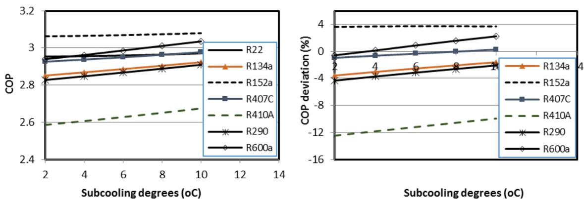
Figure 10. Variation of refrigerants' COP with subcooling degree
