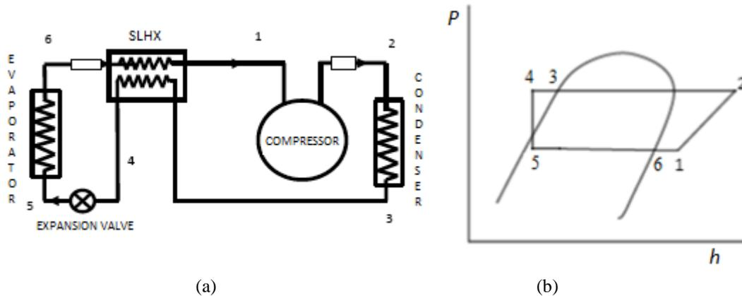
**Figure 1.** Schematic and P-h diagrams of the VCR cycle with a suction-line heat exchanger (Adapted from Venkataiah and Rao [15])
