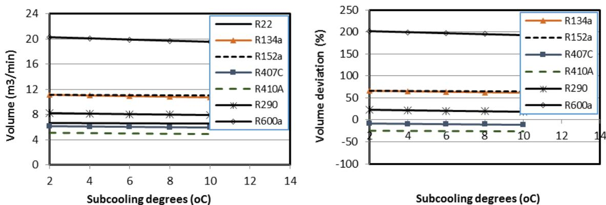
Figure 6. Variation of refrigerants' volume flow rates at the compressor inlet with subcooling degree
