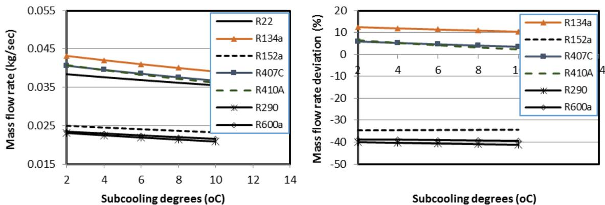
Figure 5. Variation of refrigerants' mass flow rates with subcooling degree
