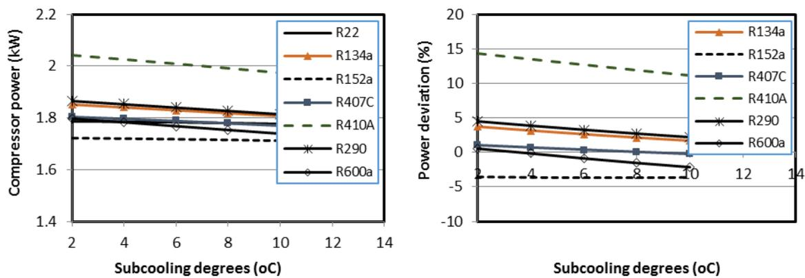
Figure 7. Variation of compressor power with subcooling degree
