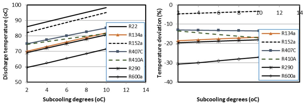
Figure 9. Variation of compressor discharge temperature with subcooling degree
