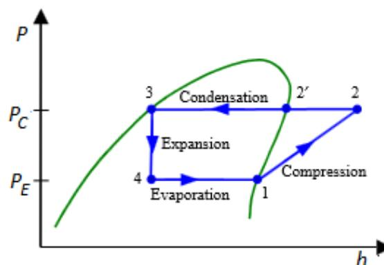
Figure 2. Ideal vapour-compression refrigeration cycle on a  $P$ - $h$  diagram (adapted from Bolaji et al [1])
