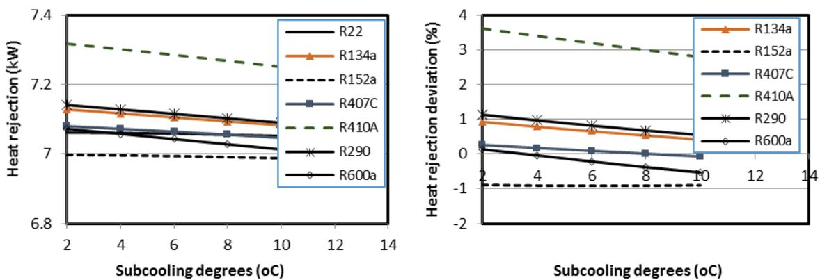
Figure 8. Variation of rate of heat rejection with subcooling degree
