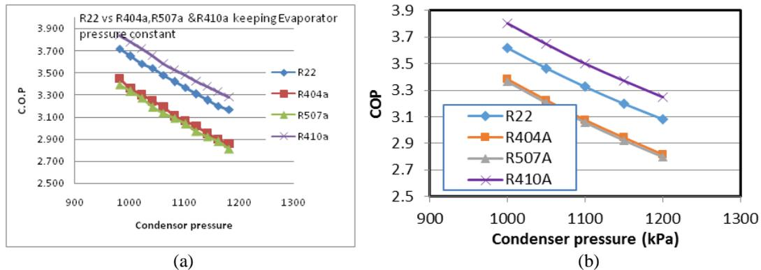
Figure 4. Variation of COP with condenser pressure: (a) Pavani et al [14], (b) present model
