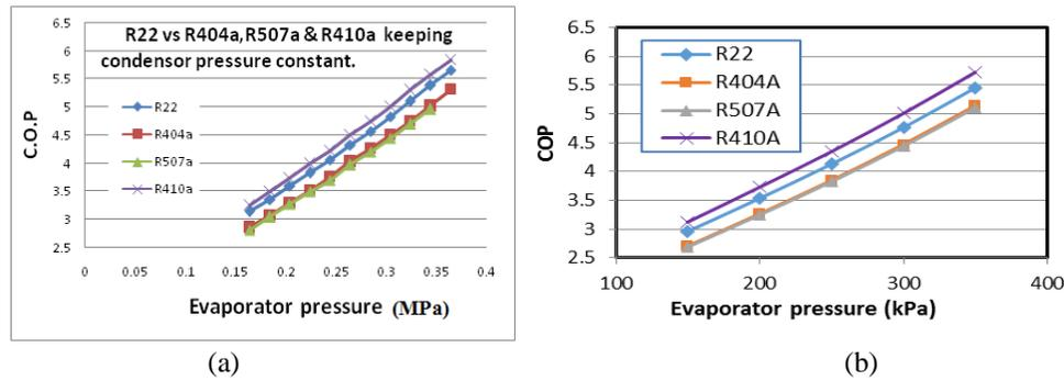
Figure 3. Variation of COP with evaporator pressure: (a) Pavani et al [14], (b) present model
