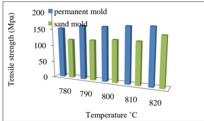
Fig.5. shows the comparison of UTS bar graph values with permanent mould and sand mould conditioned samples.
