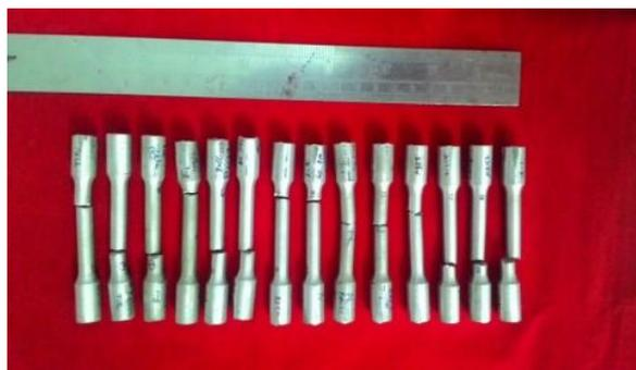
Fig.1.b. Sand mould specimens after testing conditions
