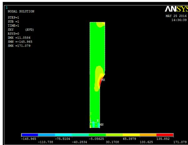
Fig: 6.b. Tensile strength distribution Sand mould in MPa
