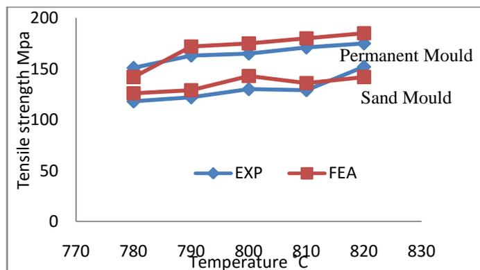
**Fig.7.** Effect of processing temperature on tensile strength of composite on FEA and Experimental results.
