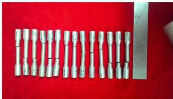
Fig.1.a. Permanent mould specimens after testing conditions
