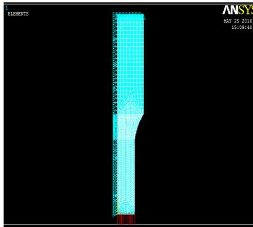
Fig.2.a. Tensile test specimen with loading and boundary condition.
