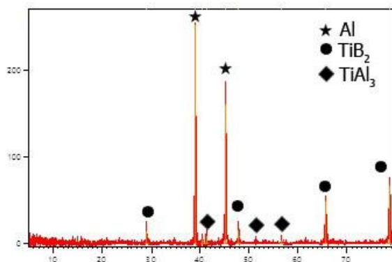
Fig.3.b. XRD graphs show the sand mould in 820°C
