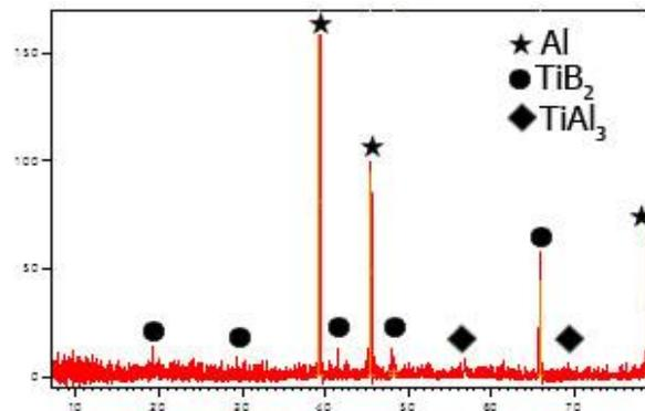
Fig.3.a. XRD graphs show the permanent mould in 820°C
