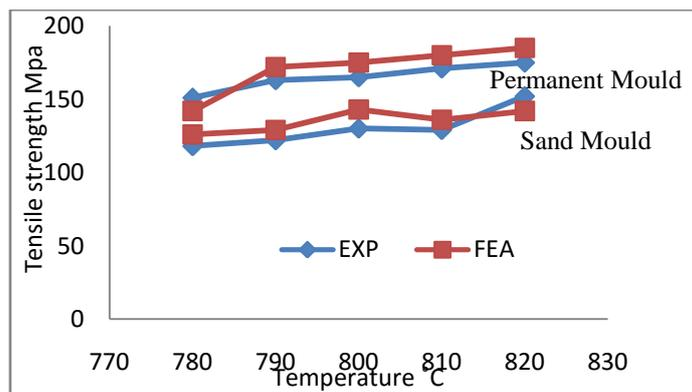
Fig.7. Effect of processing temperature on tensile strength of composite on FEA and Experimental results.
