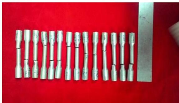
Fig.1.a. Permanent mould specimens after testing conditions
