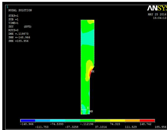
Fig: 6.a. Tensile strength distribution of permanent mould inMPa
