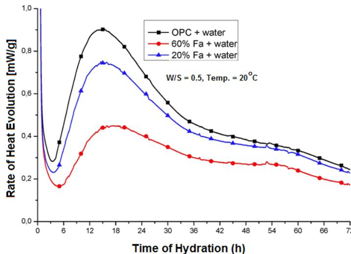
Fig. 2 Rate of heat evolution with time
