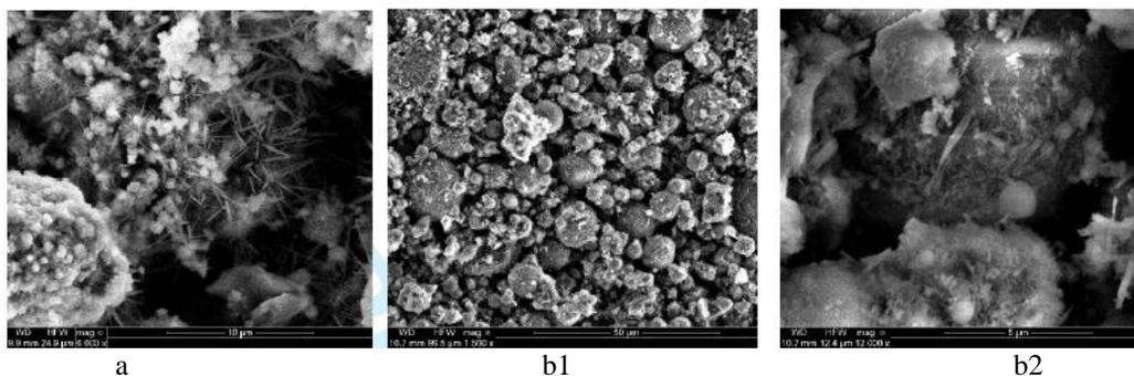
Fig.5 SEM micrograph of (a) PC hydrated for 3 d and (b1&b2)PC+60%FA hydrated for 3 d at two magnifications
