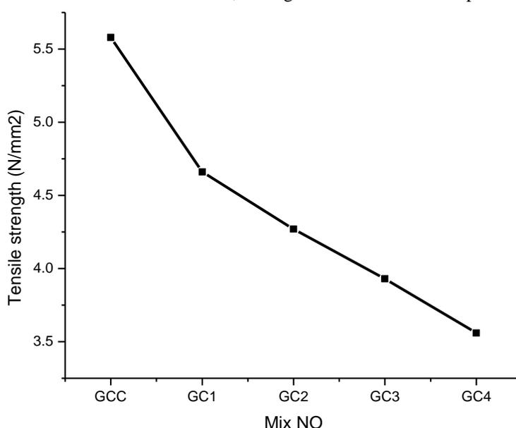
**Fig.7** Tensile Strength of OPC Concrete with Different Proportions of Fly Ash
