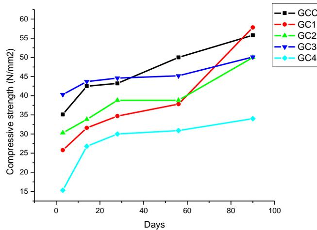
Fig.6 Compressive Strength of Concrete with Various Proportions of Fly Ash
