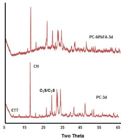
Fig.4 X-ray diffraction
