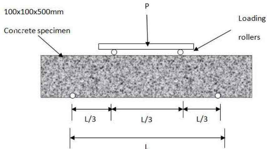
**Fig.1.** Loading Arrangement for 3-Point Flexural Test
