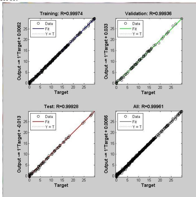
**Fig7.** Regression analysis for training, validation and test of data network.
