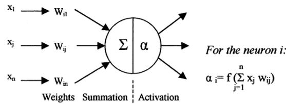
**Fig1:** the performance way in a neuron of neural network.
