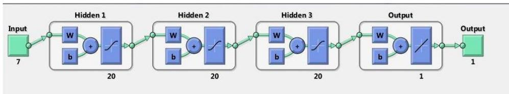
**Fig6.** The designed neural network structure.
