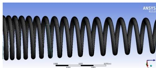
Fig. 1 Meshing of spring
