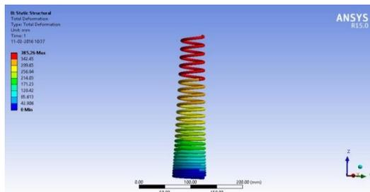
Fig. 8 Total deformation
