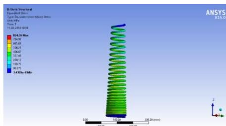
Fig.13 Equivalent stress
