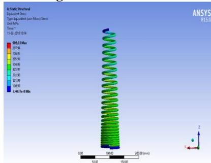
Fig. 5 Equivalent stress
