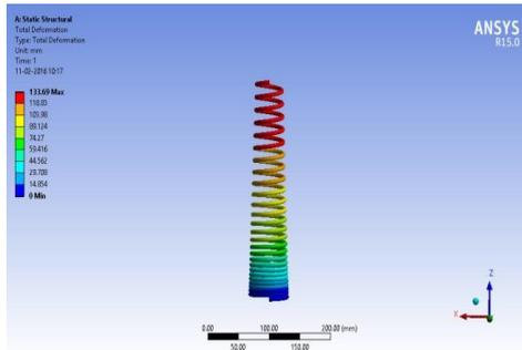
Fig. 4 Total deformation
