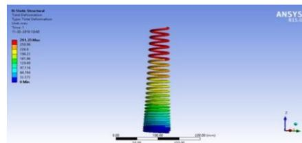
Fig.12 Total deformation
