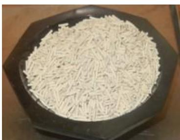
Fig 3. ZSM-5 Zeolite pellets
