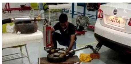
Figure 2. Setup of the reactor chamber system
