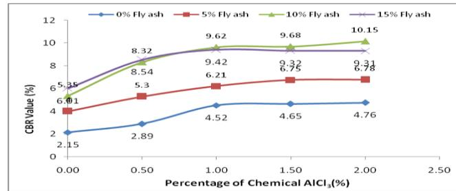
Fig. 11 Variation of California Bearing Ratio for Expansive Soil with Different % of AlCl<sub>3</sub> and Flyash.
