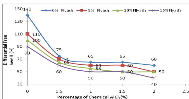
Fig. 8 Variation of Differential Free Swell for Expansive Soil with Different % of AlCl<sub>3</sub> and Flyash Mixes.
