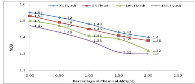
Fig. 10 Variation of Maximum Dry Density for Expansive Soil with Different % of AlCl<sub>3</sub> and Flyash Mixes.
