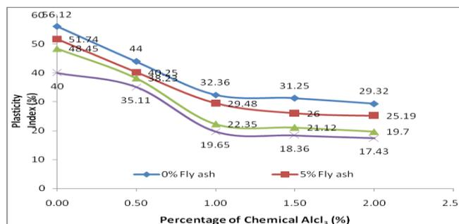
Fig. 6 Variation of Plasticity index for Expansive Soil with Different Percentages of  $AlCl_3$  and Flyash Mixes.
