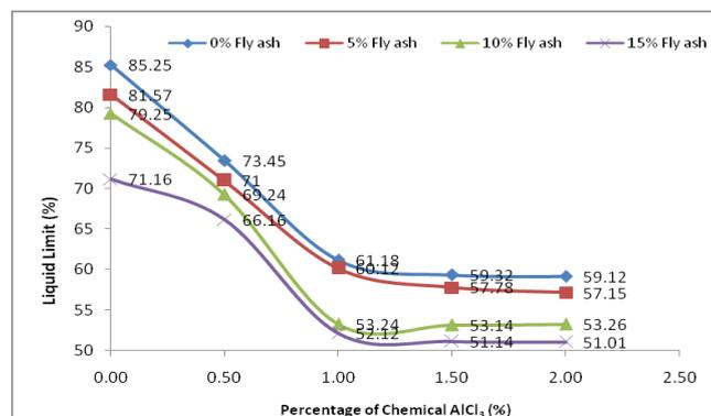
Fig. 4 Variation of Liquid Limit for Expansive Soil with Different Percentages of  $AlCl_3$  and Flyash Mixes.
