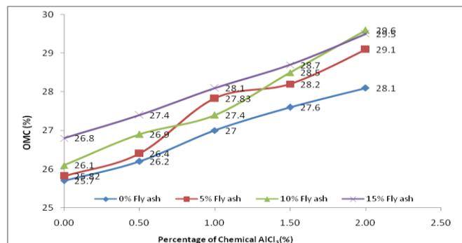
Fig. 9 Variation of Optimum Moisture Content for Expansive Soil with Different % of AlCl<sub>3</sub> and Flyash Mixes.
