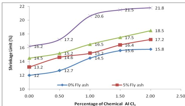
Fig. 7 Variation of Shrinkage Limit for Expansive Soil with Different Percentages of AlCl<sub>3</sub> and Flyash Mixes.
