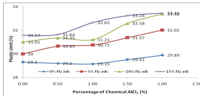
Fig.5 Variation of Plastic Limit for Expansive Soil with Different Percentages of  $AlCl_3$  and Flyash Mixes.
