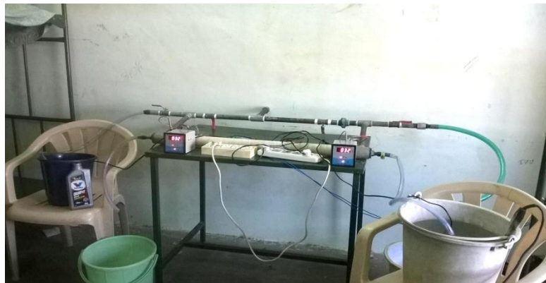
Fig No.1. Experimental Set-Up of Counter Flow Heat Exchanger
