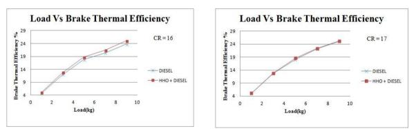
Fig. 9 Load Vs Brake Thermal Efficiency at CR 16 Fig. 10 Load Vs Brake Thermal Efficiency at CR 17
