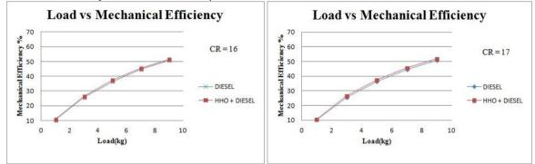
Fig. 12 Load Vs Mechanical Efficiency at CR 16Fig. 13 Load Vs Mechanical Efficiency at CR 17
