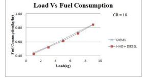
Fig. 5 Load Vs Fuel Consumption at CR 18
