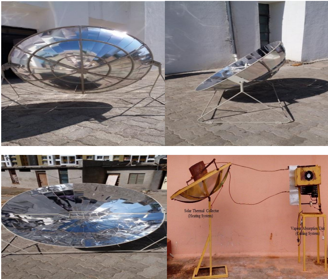
Fig.1 (b) Experimental set-up of Solar cooling System
