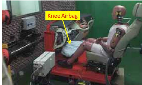
Fig. 1: Knee Airbag with Crash Dummy and Sled Environment [5]
