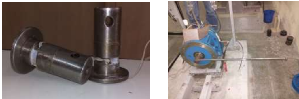
Fig. 2 Strain Gauge Location And Loading Setup For Static Measurement
