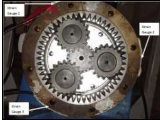
Fig. 22 Strain Gauge Location On The Rim Of The Ring Gear.
