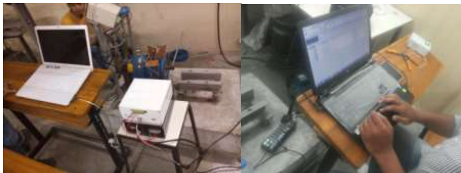
Fig. 4 Panopticonode J-Logger And DEWE 43 Setup
