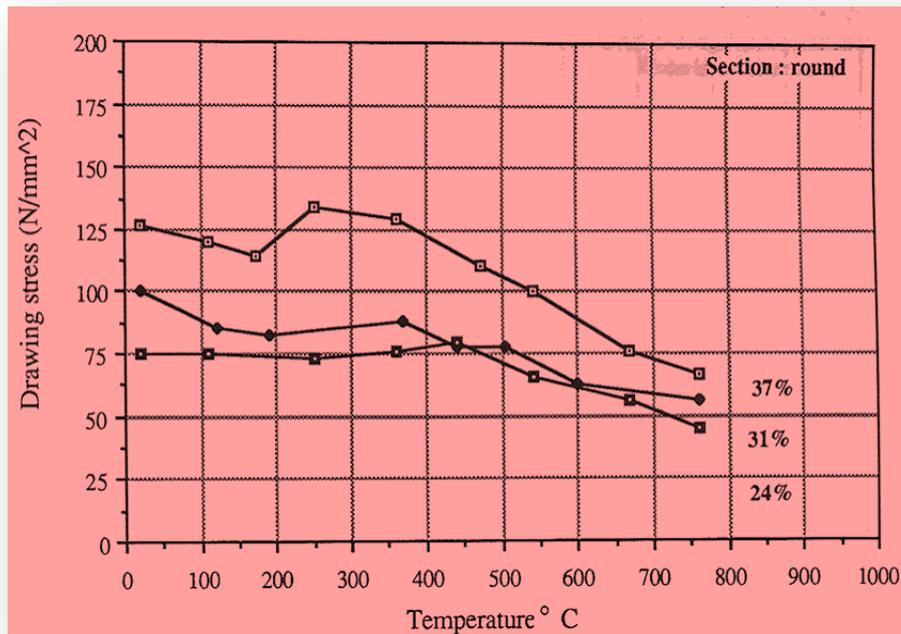
Fig 3.3. Variation of experimental drawing stress with temperature and reduction of area using Tungsten carbide dies.
