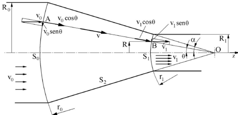
Fig. 2.1 Model of the Velocity field Assumed in Avitur's Theoretical Model of Wire Drawing Process (1997).
