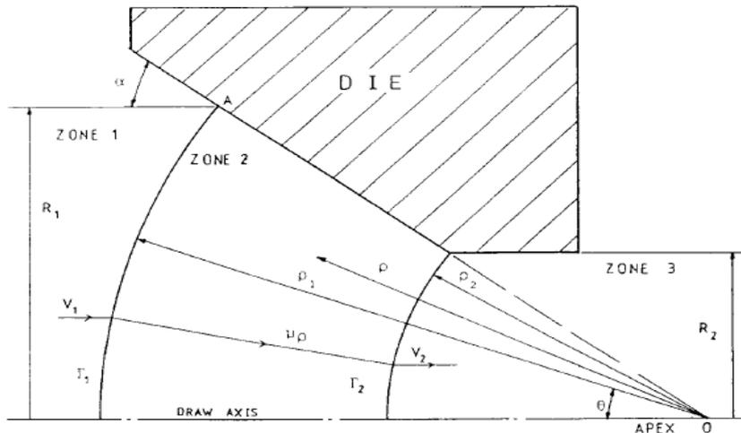
Fig. 3.2 Model of Velocity Flow ( $\rho_0 = OA$ )
