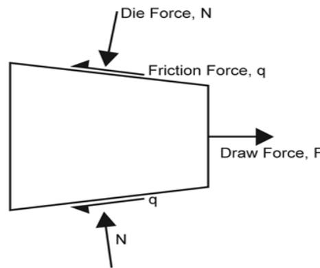
**Fig.2.4 Free body diagram showing primary forces in wire drawing**
