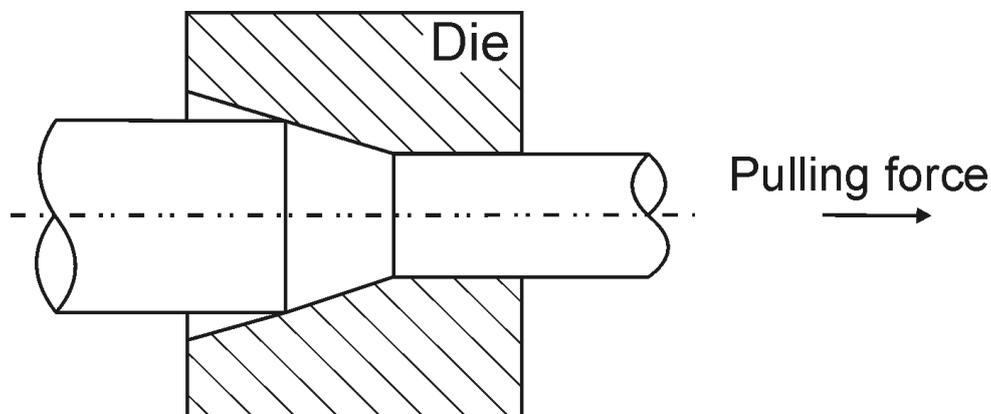
Fig. 2.2 Wire Drawing Concept
