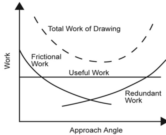
**Fig. 2.3 Components of work that operate during wire drawing**
