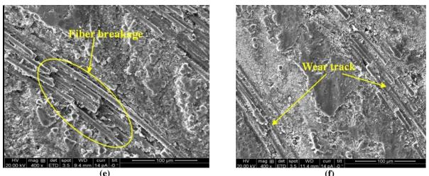
Figure 9: SEM pictures of composites for bone powder filled hybrid composites
