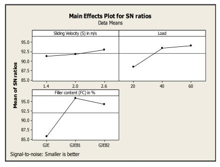
Figure 1: Effect of control factors on specific wear rate of hybrid composites
