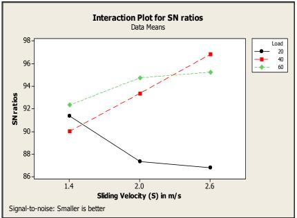
Figure 3: Interaction graph between sliding velocity and normal load for specific wear rate
