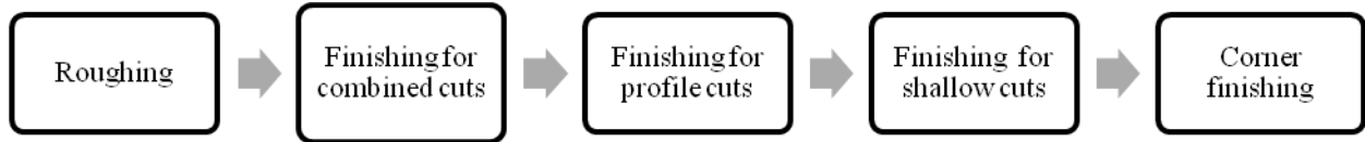
Figure 5 Operations considered for generating NC program for cavity
