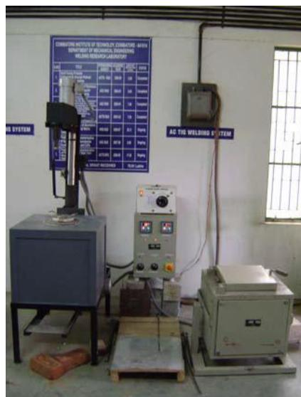
Stir casting furnace setup
