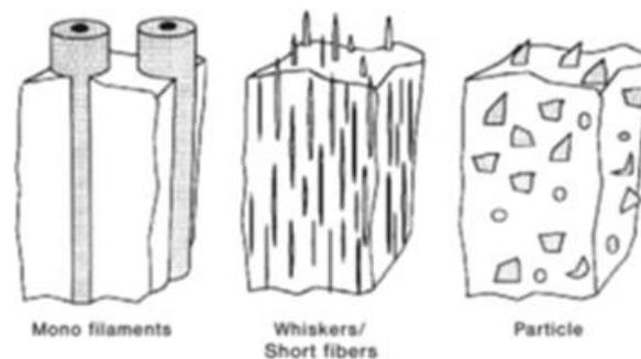
Fig. 2.3: Schematic presentation of three shapes of metal matrix composite materials [15]
