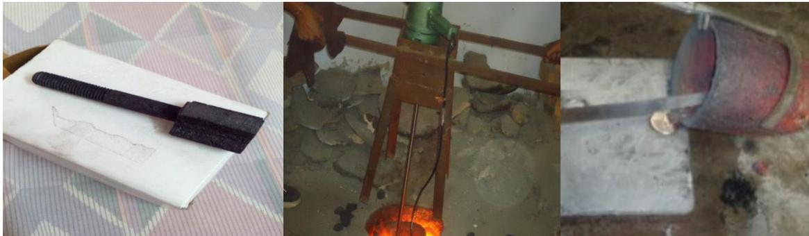
Graphite Stirrer Stirring of Al+ SiC mixture using motor Pouring of molten Al into mould
