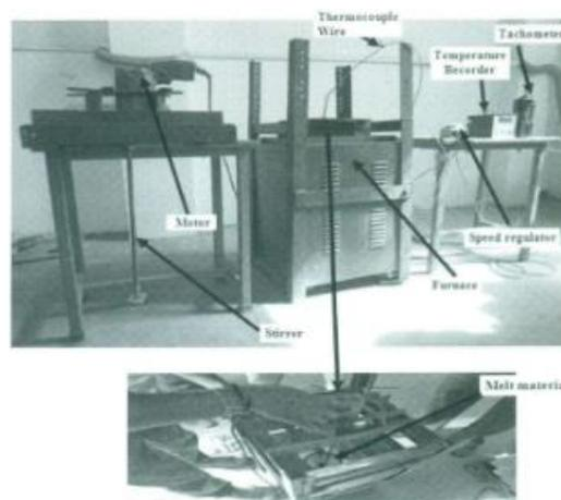
Experimental setup of mechanical stir casting
