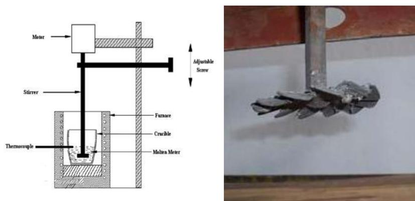
Schematic view of Experimental setup and stirrer
