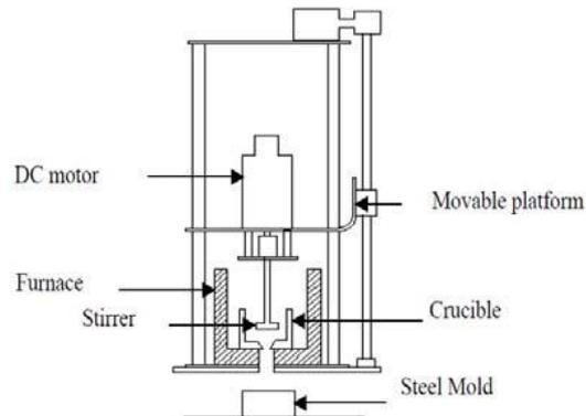
Schematic drawing of the utilized rheocaster device
