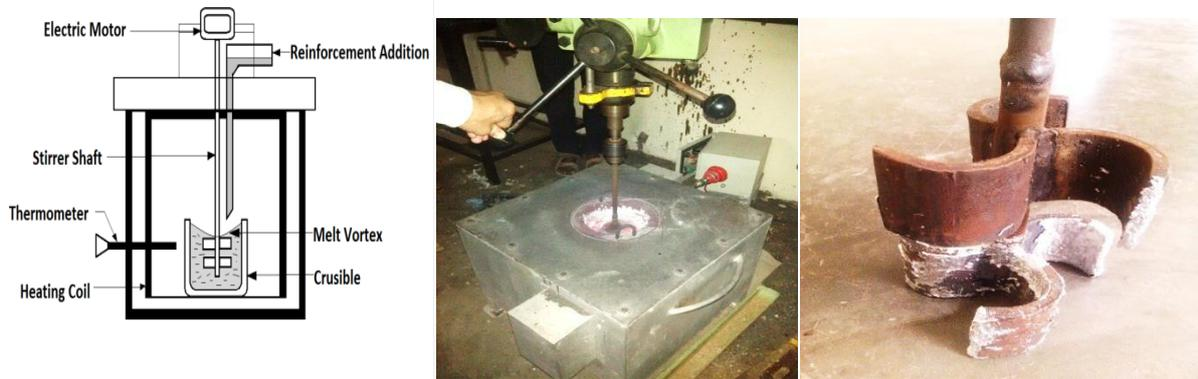
Stir Casting Setup (Schematic) Stirring process Stirrer Blades
