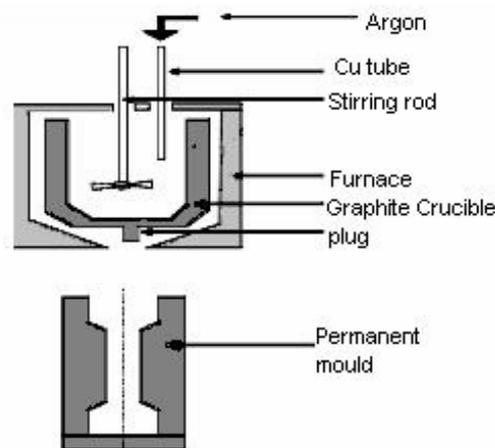
Schematic diagram experimental stir cast set-up
