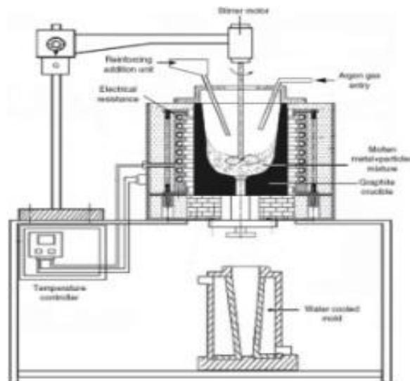
Fig. 3.2: Stir casting machine (equipped with inert gas source and pour molten system)[22]
