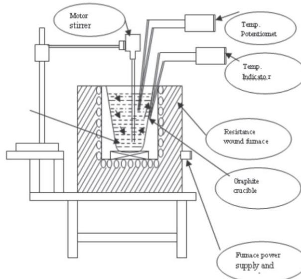
Schematic representation of stir casting set-up
