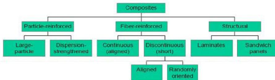
Fig. 2.2: classification scheme for the types of composites[11]
