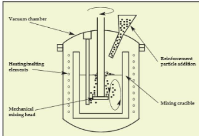
Fig. 3.1: Conventional stir-casting setup for the compositing of aluminum MMC material. This is the most common commercial method. [21]
