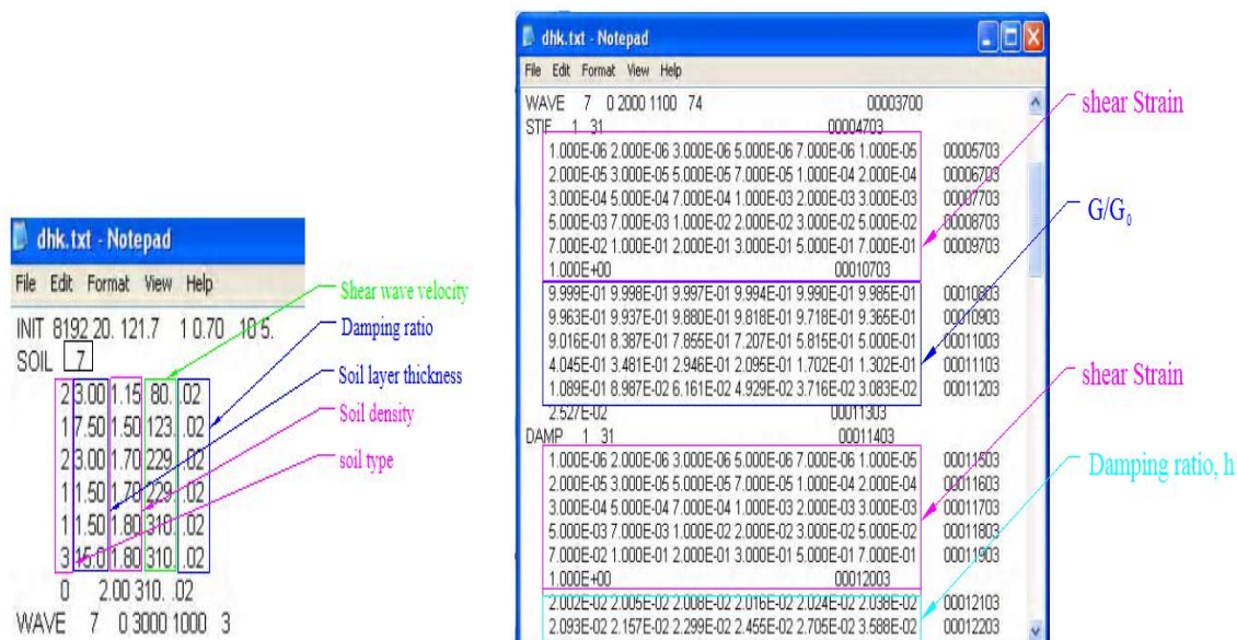
Fig.14 Input data of soil properties.
