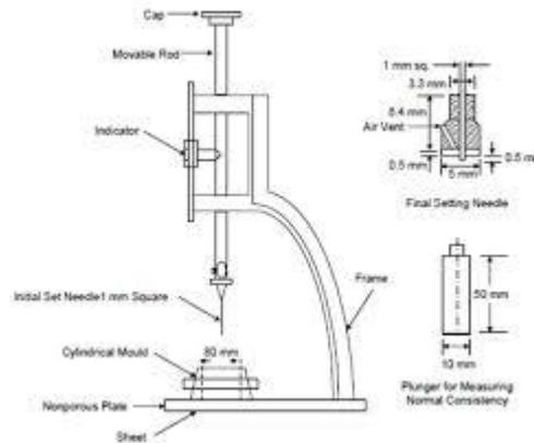
Standard consistency, initial setting time, final setting time and compressive test for cement should confirm Indian Standards 4031 (Part 4 to Part 6).
