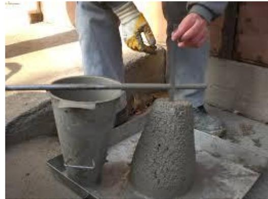
**Flow Test:** Flow test is generally used for highly workable concrete. Flow of concrete can be measured by flow table. Workability of Ready Mix Concrete should be maintained as per demand of purchaser and environmental conditions given in Indian standard 456:2000 clause no. 7.1.
