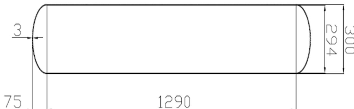
Figure 8- Geometrical model of the bottle the 35K
