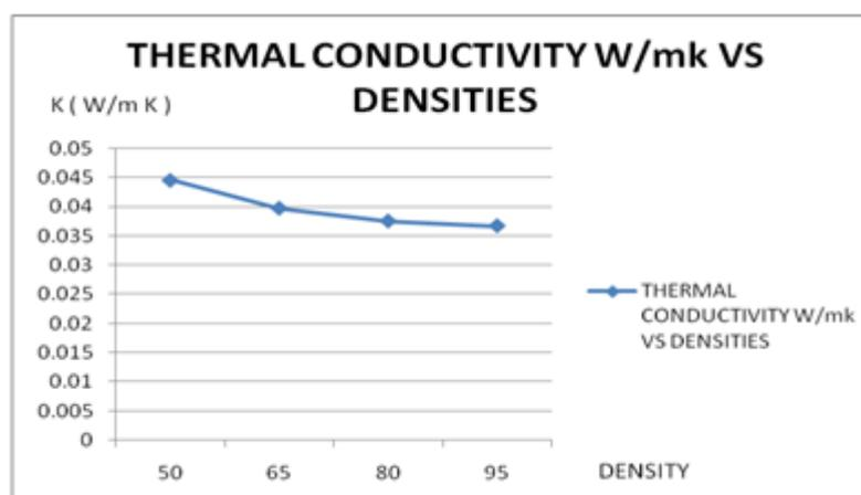
**Graph 1:** Thermal Conductivity Vs Densities of Coconut Fibre
