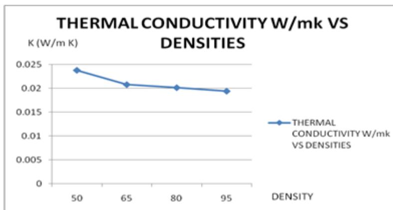
**Graph 3:** Thermal Conductivity Vs Densities of polyurethane
