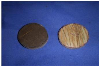
Fig.1 Coconut Fibre Sample
