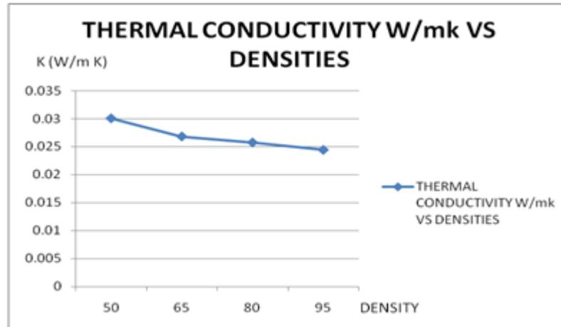
**Graph 2:** Thermal Conductivity Vs Densities of polystyrene
