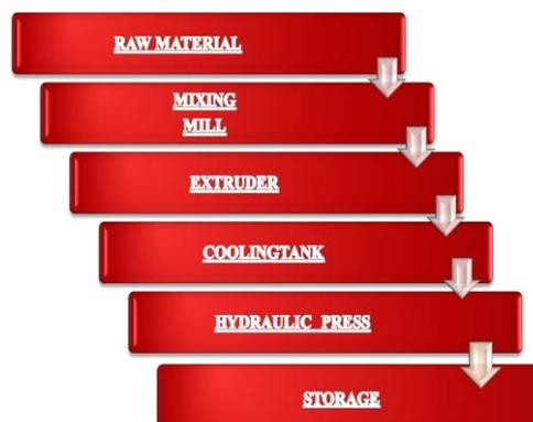
Fig 5 Manufacturing Sequence for Cold or Pre-cured Tread Rubber
