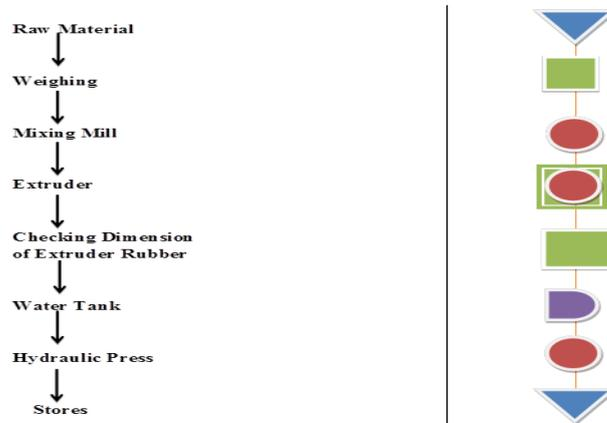
**Fig 9** Outline Process Chart for Cold Tread Rubber
