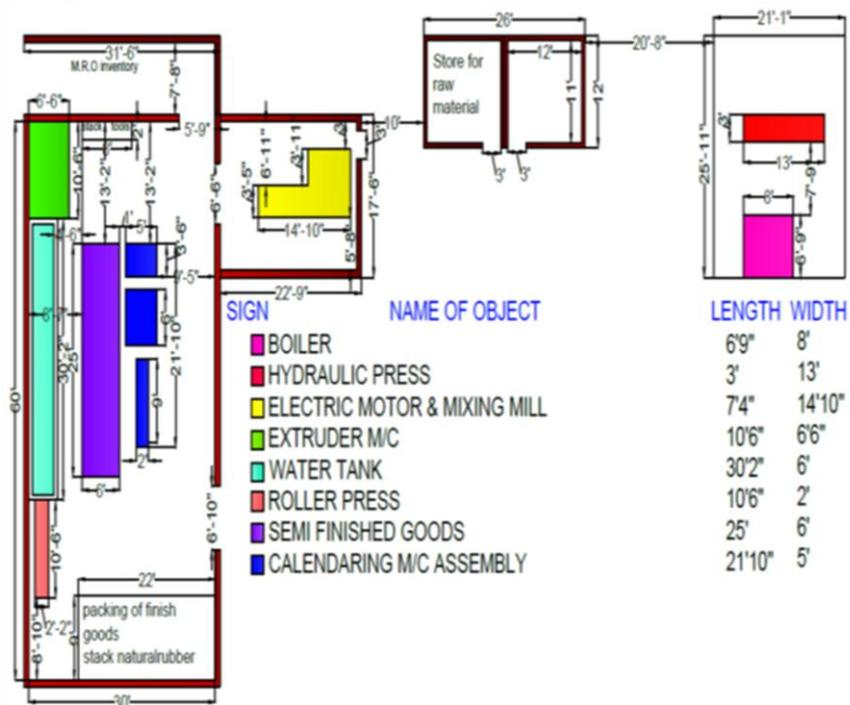
Fig 6 Existing Plant Layout of C.R.P at G.I.D.C
