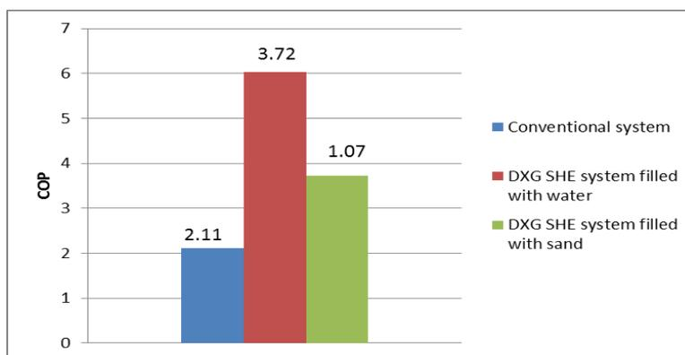
**Fig. 4. The comparison of COP of Conventional Air condition system, ACSWGSHE filled with water and ACSWGSHE filled with sand.**
