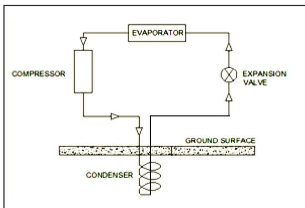
Fig.1. Schematic diagram of ACSWGSHE system
