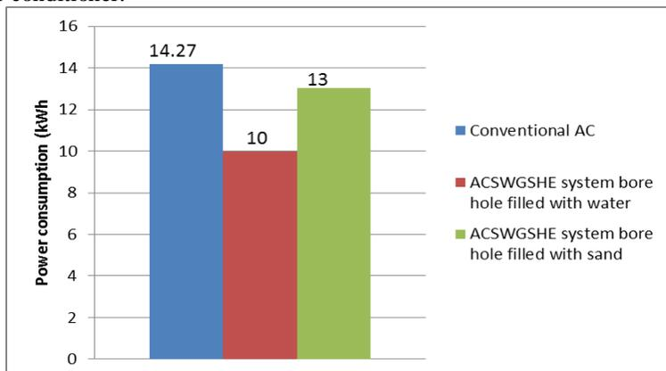
**Fig. 3. The comparison of Power consumption of Conventional Air condition system, ACSWGSHE filled with water and ACSWGSHE filled with sand.**
