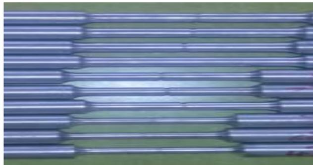
Fig. 2. Circumferentially crack round bar testing specimens
