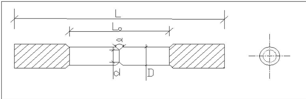
Fig. 1. Schematic representation of round notched tensile specimen
