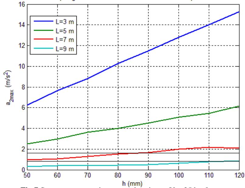
Fig.7 Sprung-mass maximum acceleration at V = 25 km/h .
