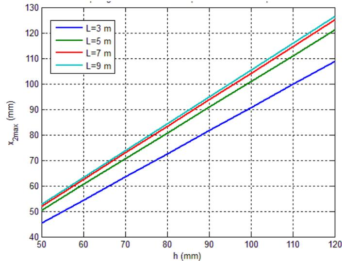
Fig.5 Sprung-mass maximum displacement at  $v = 25$  km/h.
