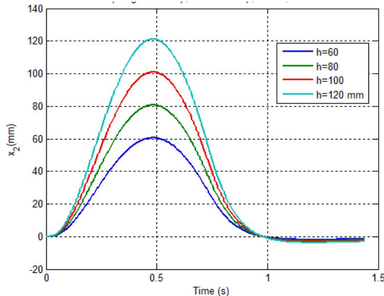
Fig.4 Sprung-mass displacement for V = 25 km/h.
