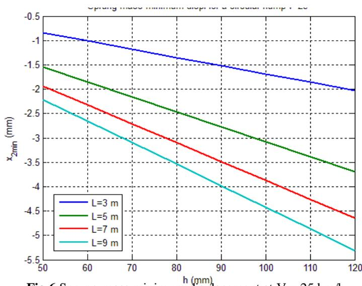
Fig.6 Sprung-mass minimum displacement at  $V = 25$  km/h.
