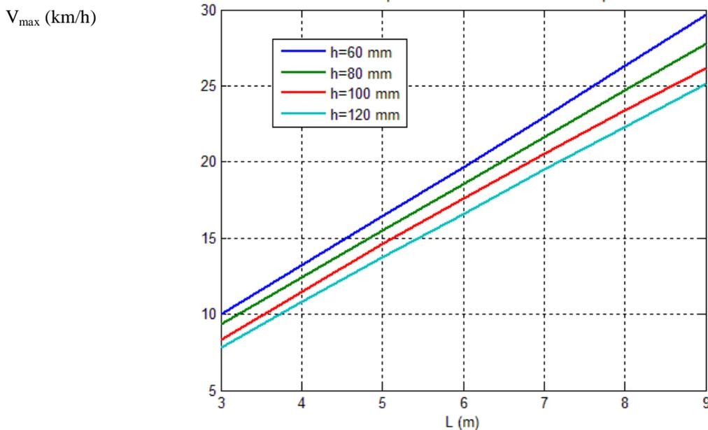
Fig.8 Car maximum speed for ride comfort across the simple harmonic hump
