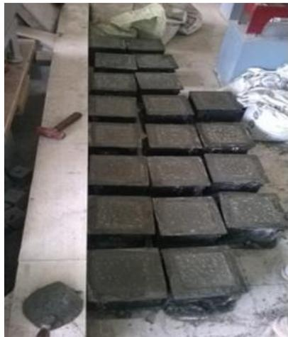
Figure 3: Casting of Cubes
