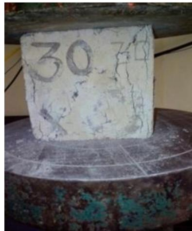
**Figure 4:** Cube compression test
