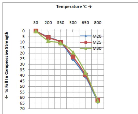
Figure 5: % Fall in compressive strength after 1 hour      Figure 6: % Fall in compressive strength after 2 hours
