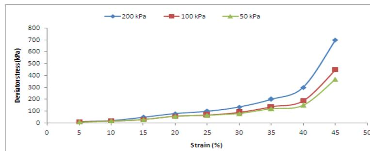
**Fig. – 5** Deviator stress-strain curves of direct shear tests.
