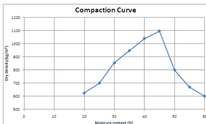
Fig -4 Dry density – moisture content curve
