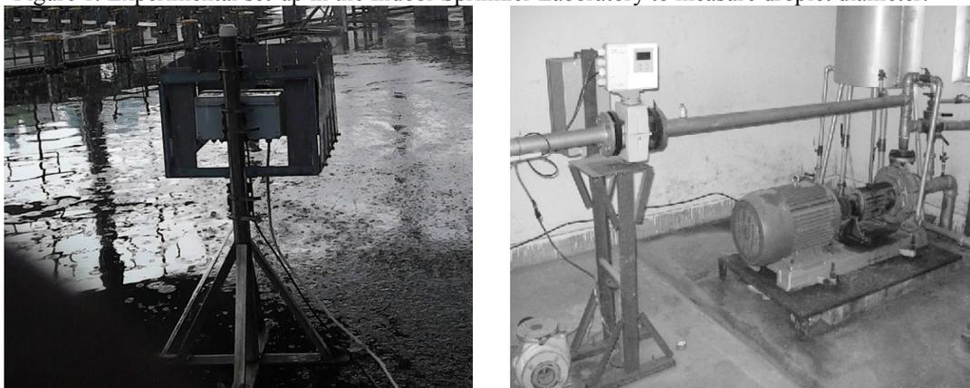
Figure 2: TCLPM instrument, Pump and Flow meter set-up in the Sprinkler Laboratory
