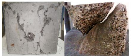
a) Mix#1 (Vertical Crushing) b) Mix#2 (Vertical Crushing + Shear) Fig. 6.failure modes of laboratory and field casted samples - compression test
