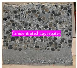
Fig. 9.illustration of segregation along concrete cross section.
