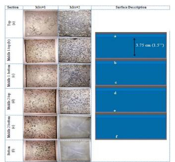
Fig. 10.cross-section investigation along depth of specimens for Mix#1 and Mix#2
