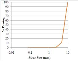
Fig. 1.gradation of as received aggregates
