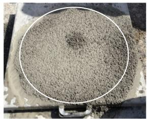
Fig. 8.slump flow – field application.
