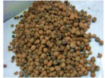
Fig. 2.sintered pulverized-fuel ash aggregates
