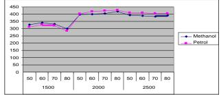
Fig.4.15 The effect of engine coolant temperature on HC emission with varying engine speed and at an engine load of 12 kg
