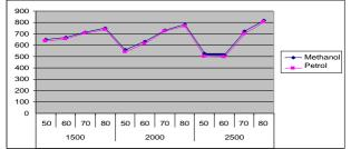
Fig.4.16 The effect of engine coolant temperature on NOx emission with varying engine speed and at an engine load of 6 kg
