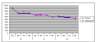
Fig.4.8 The effect of engine load on specific fuel consumption with varying engine coolant temperature and at an engine speed of 2000 rpm
