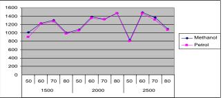
Fig.4.17 The effect of engine coolant temperature on NOx emission with varying engine speed and at an engine load of 9 kg
