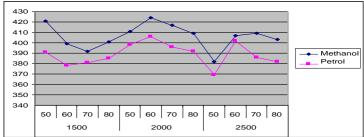
Fig.4.14 The effect of engine coolant temperature on HC emission with varying engine speed and at an engine load of 9 kg
