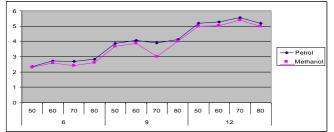
Fig.4.11 The effect of engine load on brake power with varying engine coolant temperature and at an engine speed of 2000 rpm
