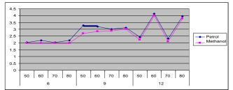
Fig.4.10 The effect of engine load on brake power with varying engine coolant temperature and at an engine speed of 1500 rpm
