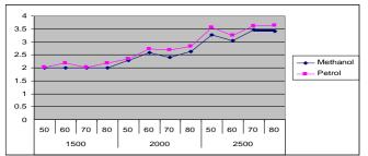
Fig.4.4 The effect of engine coolant temperature on brake power with varying engine speed and at 6 kg engine load.
