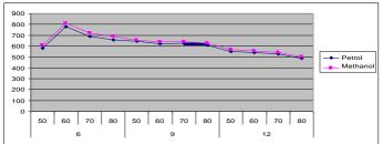
Fig.4.9 The effect of engine load on specific fuel consumption with varying engine coolant temperature and at an engine speed of 2500 rpm
