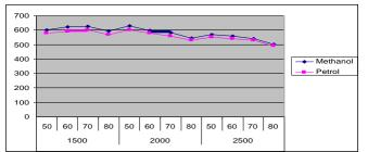
Fig.4.3 The effect of engine coolant temperature on specific fuel consumption with varying engine speed and at 12 kg engine load.
