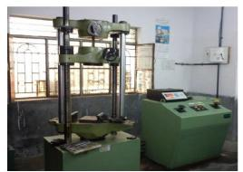
Figure 1: Universal Testing Machine
