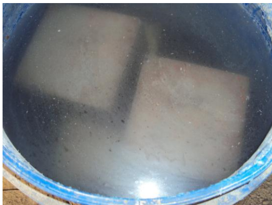
Plate 5: Curing of the concrete cubes by immersion
