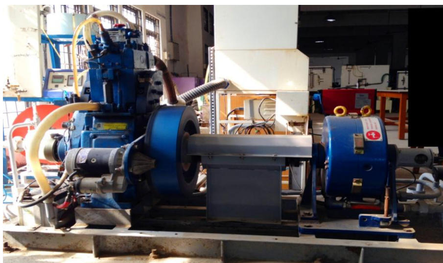
Fig.2 Photographic view of single cylinder four stroke diesel engine
