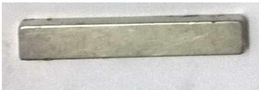
Fig.4 Photographic view of Neodymium Magnets
