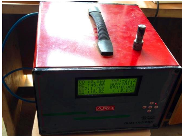
Fig.3. Photographic view of exhaust gas analyzer
