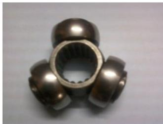
Figure 3–Tripod assembly.
