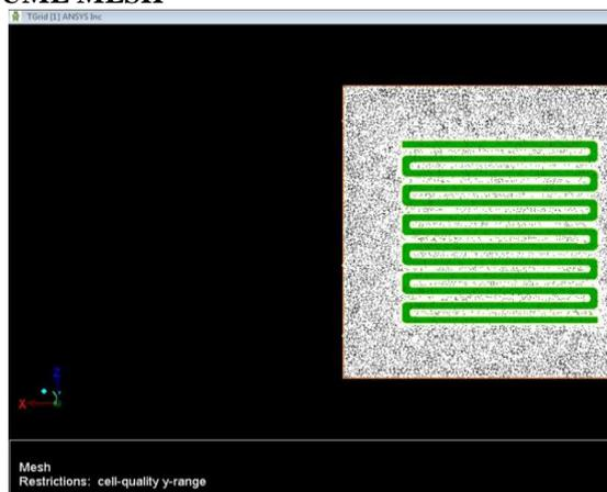
Figure 6 volume meshing in T-grid
