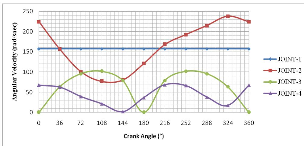
*Fig-14: Plot of angular velocity of revolute joint (1500 rpm crank speed)*
