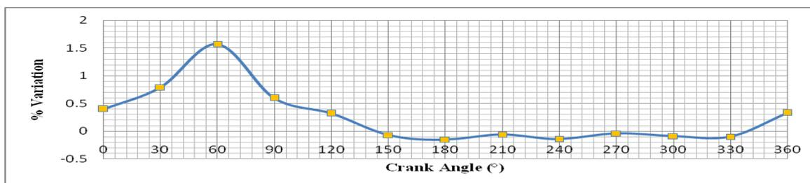
Fig-19: Plot of variation in maximum angular velocity of coupler (1500 rpm crank speed)
