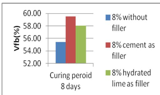
Fig.21 Curing period vs. Vfb
