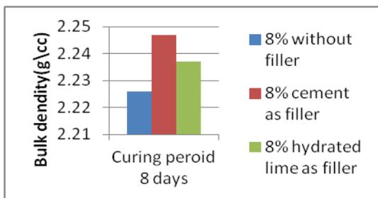
Fig.19 Curing period vs. Bulk density
