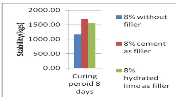
Fig.23. Curing period vs. stability
