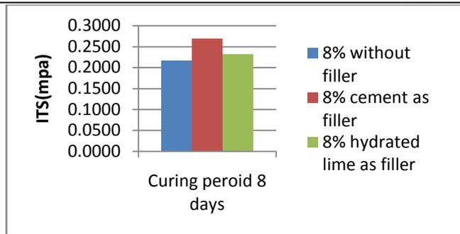
Fig.25 Curing period vs. ITS (mpa)
