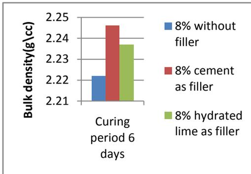
Fig. 6 curing period vs. Bulk density
