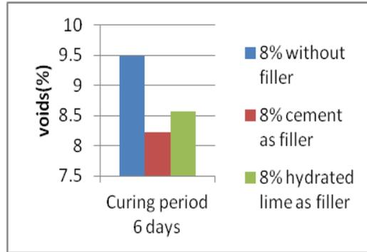
Fig. 7 Curing period vs. voids in total mix
