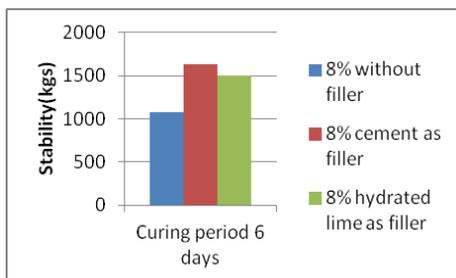
Fig.10 curing period vs. Stability
