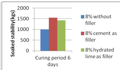
Fig.11 Curing period vs. soaked stability
