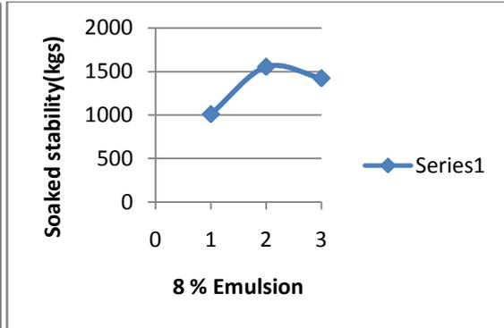
Fig. 5 Soaked stability vs. Emulsion without and with filler
