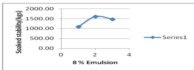
Fig. 18 Soaked Stability vs. Emulsion without and with filler
