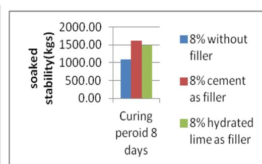
Fig.24 Curing period vs. soaked stability
