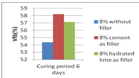
Fig. 8 Curing period vs. voids filled with bitumen
