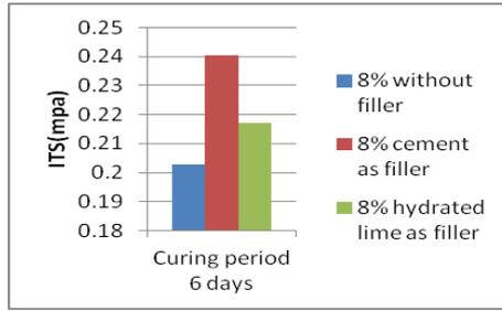
Fig..12 curing period vs. ITS
