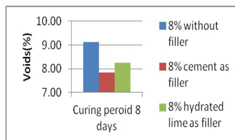
Fig.20 Curing period vs. Voids
