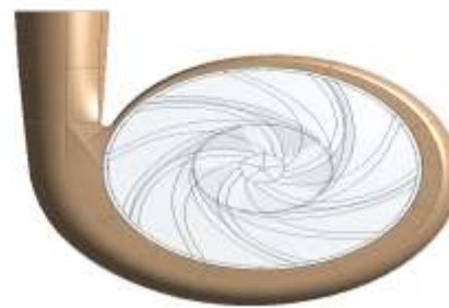
Fig. 2 Geometric model pump with volute casing
