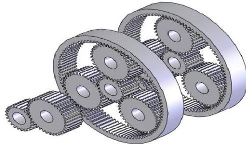
Fig.4a -Traditional Wind Turbine Gearbox
