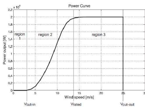
Fig1. Power o/p Vs Wind speed
