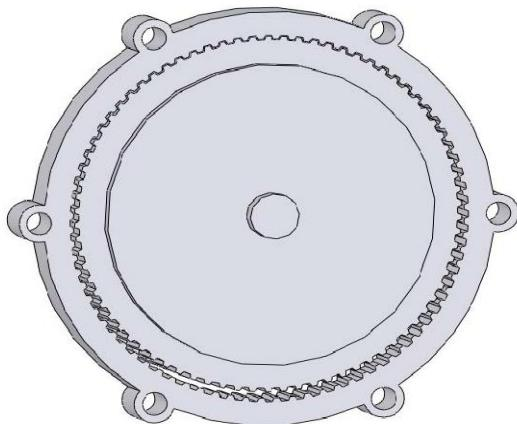
Fig. 14-Torque Distributed Over Several Gear Teeth
