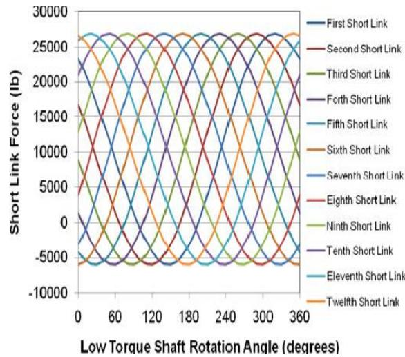
Fig. 13-Short Link Forces for One Rotation of the Low Torque Shaft
