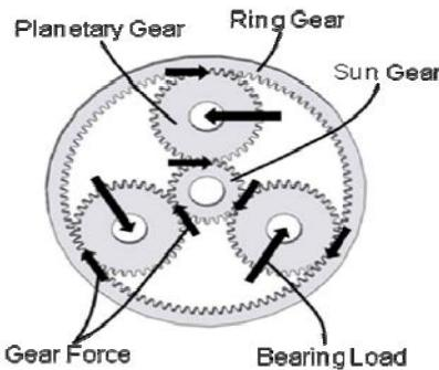
Fig 4b.-Planetary Gear Set Loads
