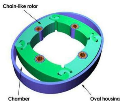
Fig.2 -QT Rotor.
