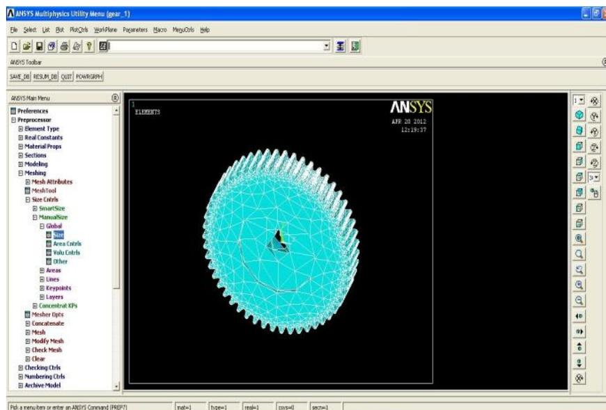
Figure No. 1 Meshing of Gear
