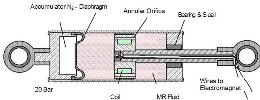
Fig.4.2 Commercial Linear MR Fluid-based Damper
