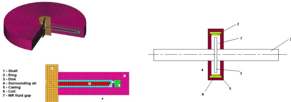
Fig.3.1 Basic configuration of the proposed MR brake
