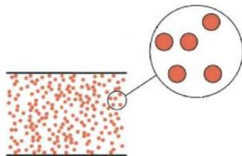
Fig.2.1 MR Fluid model without outer magnetic field
