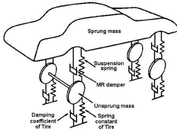
Fig.4.1 the Model of Vehicle
