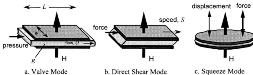
Fig.2.3 the three basic work modes of MR Fluid devices
