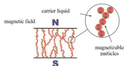
Fig.2.2 MR Fluid model in outer magnetic field
