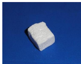
Figure 3.1 Scaffold prepared by Polymeric Sponge Method
